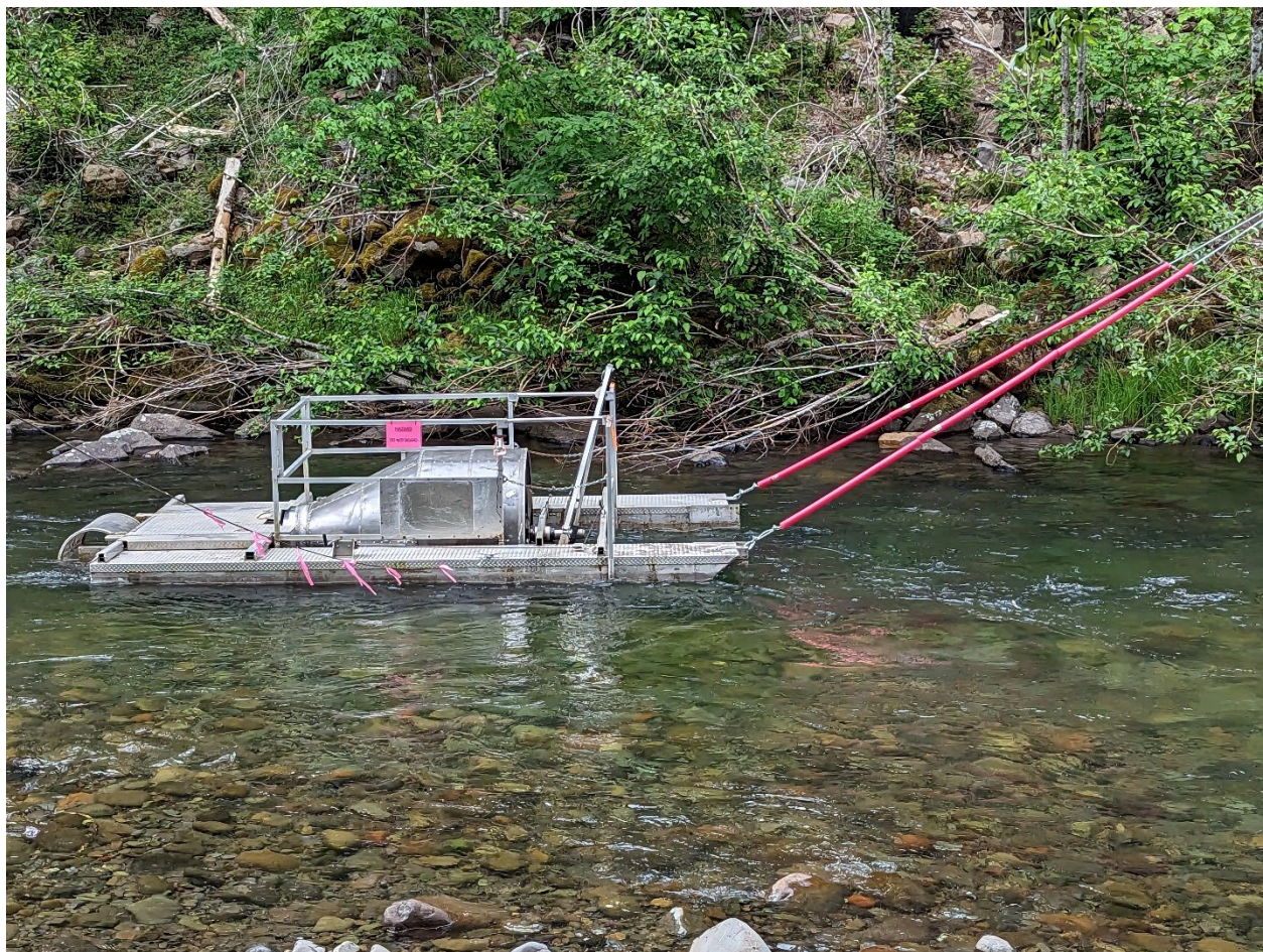
Figure H-2. RST sampling at the Breitenbush River site in low flow.
