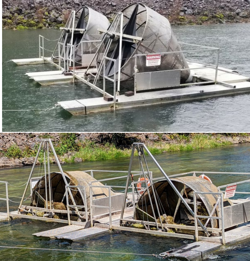
Figure H-10. Cougar Dam – Powerhouse Channel when not sampling (above) and when sampling with high debris (right).
