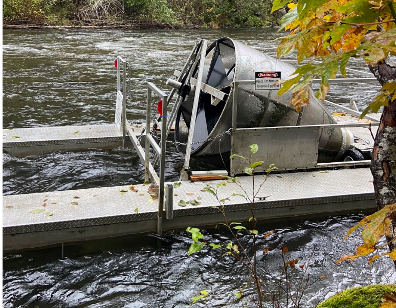
Figure H-8. Cougar Dam Head of Reservoir not sampling at high flow.
